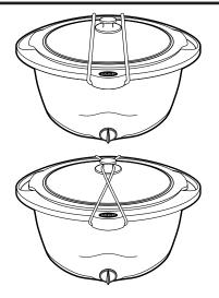
The **Lid Latch** secures the cover while moving, transporting, or storing the slow cooker. To use the Lid Latch, place the white band under the tab at the front edge of slow cooker base. Stretch the band to the other side of the slow cooker and secure it in the same way.
